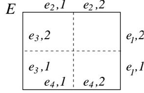
Figure 8. An element,  $E$ , the local edges,  $e_1$  to  $e_4$ , and the sub-edges  $e_k$ , for  $i = 1, \dots, 4$ , and  $k = 1, 2$ .
