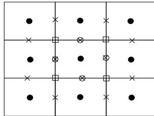
Figure 4. Computational molecule for CCFDM in the reference space, showing  $p$  (solid dots),  $\mathbf{u}$  (open circles),  $\tilde{\mathbf{u}}$  (crosses), and the evaluation of  $\mathbf{K}$  (boxes at vertices).
