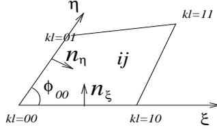
Figure 12. One SOM element, with the local coordinates for the element vertex  $kl = 00$
