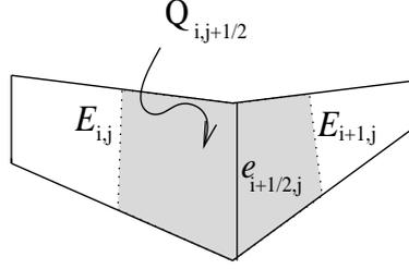
Figure 2. Two adjacent gridcells, and the area of support for the velocity function,  $Q_{i,j+1/2}$
